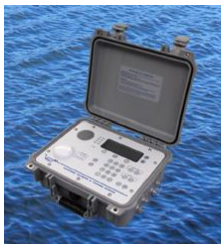
Figure C-1: Testing the detection range (m) of an acoustic tag in Te Waihora using two different detection devices. The tag being tested was a high power V13 tag manufactured by VEMCO. The tag was placed on the bed of the soft-bottomed lake at a depth of 0.7m. The different devices used for tag detection are shown below. The VR100 hydrophone is typically used for real-time detection whereas the VR2W receivers are the devices left in place in the lake for continuous monitoring. The testing was undertaken at Timber Yard Point.
