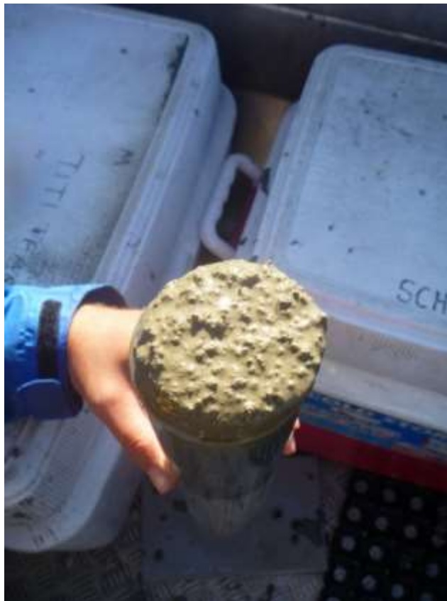
Sediment core collected at site E18, containing chironomid tubes.
