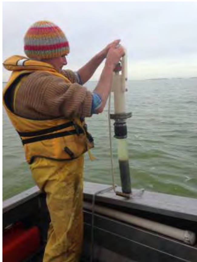
Collecting a sediment core using a gravity corer.
