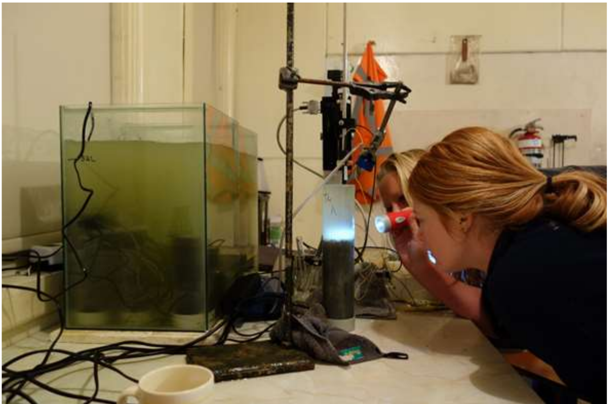
Measuring sediment oxygen micro-profiles using a Unisense oxygen microsensor.
