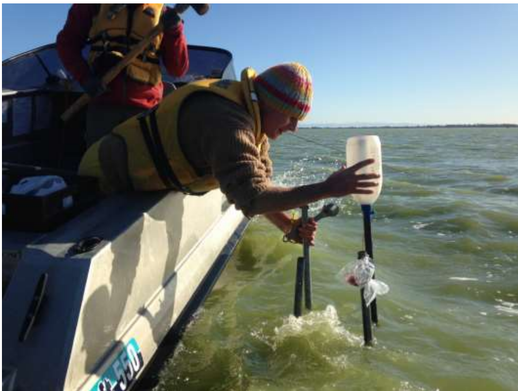
Setting up the in situ denitrification enclosure.
